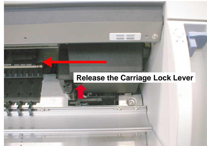
Figure 4-83. Releasing the CR Lock Lever
