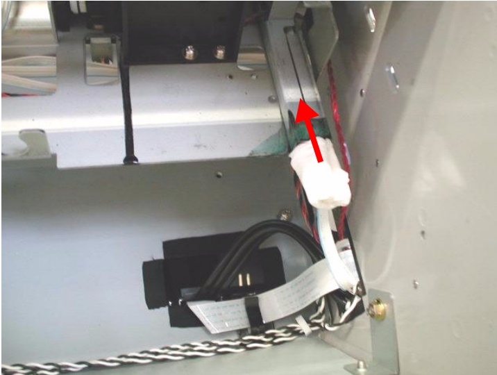
Figure 4-81. Preventing the Leakage of Ink from the Waste Ink Tubes
