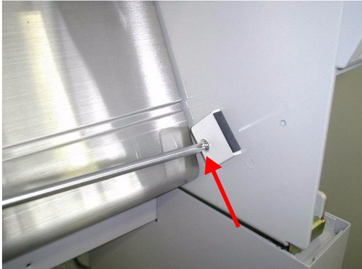
Figure 4-73. Removing the Right Cover Holder Assembly
