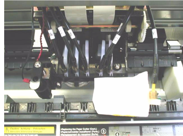
Figure 4-94. Removing the Dampers
