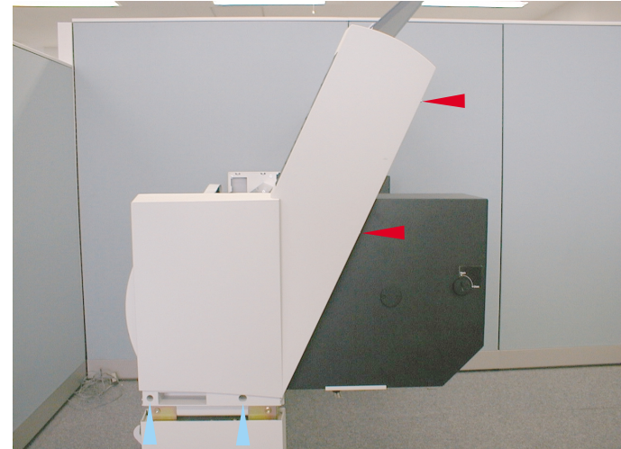
Figure 4-72. Removing the Right Side Frame
