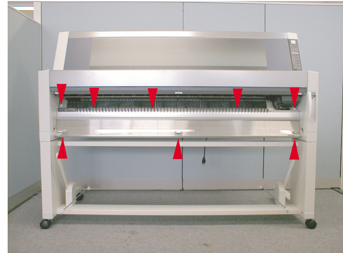
Figure 4-75. Removing the Paper Guide L (1)
