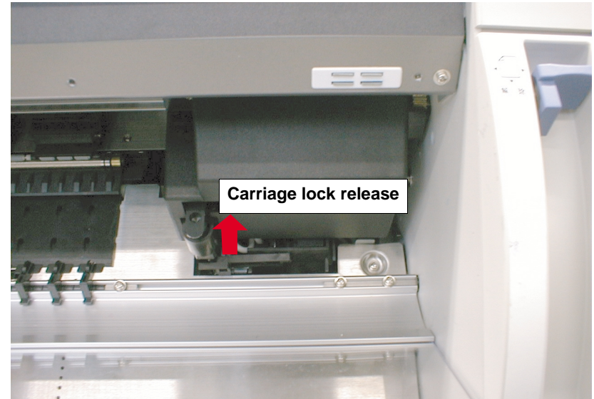
Figure 4-20. Carriage Lock Release
